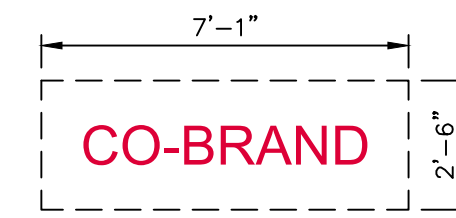
D PROPOSED CO-BRAND SIGN AREA=17.7 S.F. (QTY. 1) NOTE: TENANT SIGN/BASE TO BE PER CO-BRAND SPECIFICATIONS
