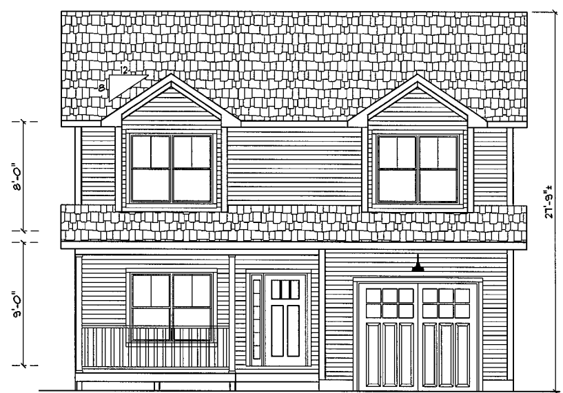
NOTE: GUARD RAILS NOT REQUIRED UNLESS DECK IS 30" ABOVE GRADE FRONT ELEVATION 1/4"=1'-0"
