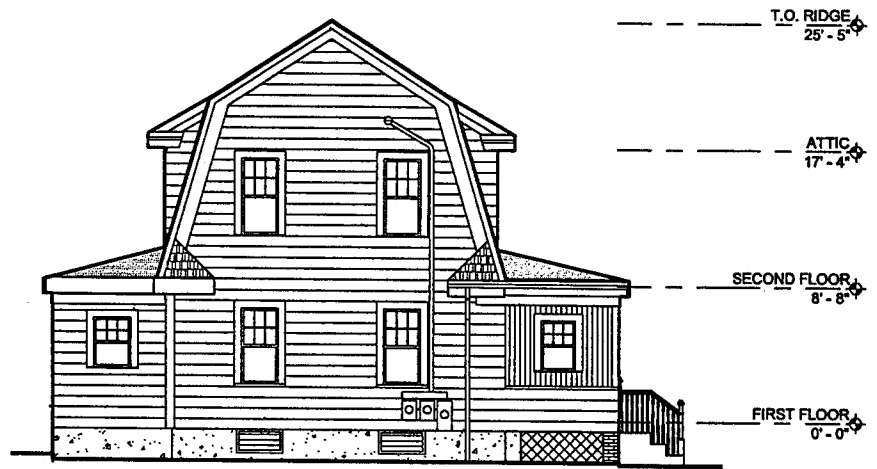
7 SIDE ELEVATION (NORTH) 1/8" = 1'-0"
