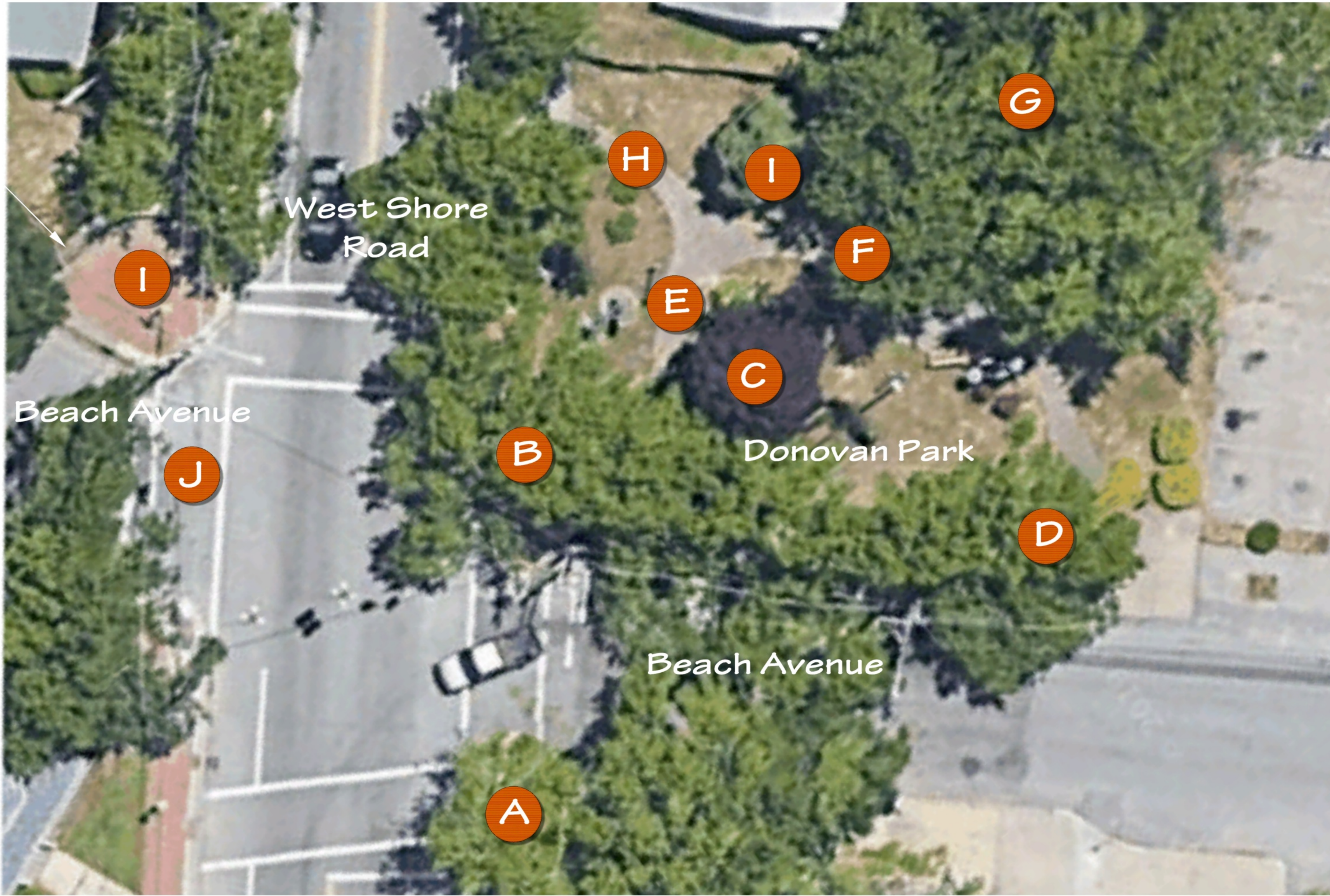
F Donovan Park - Remove existing concrete pavers and seal. Reset existing granite seal. Install new 4"X8" brick pavers to match bricks on West Shore Road. Infill with gray polymeric sand. Seal brick with Techniseal ProSeries Waterproofing Sealant for Brick and Concrete (WR7) or approved equal. Apply according to manufacturer recommendations.
