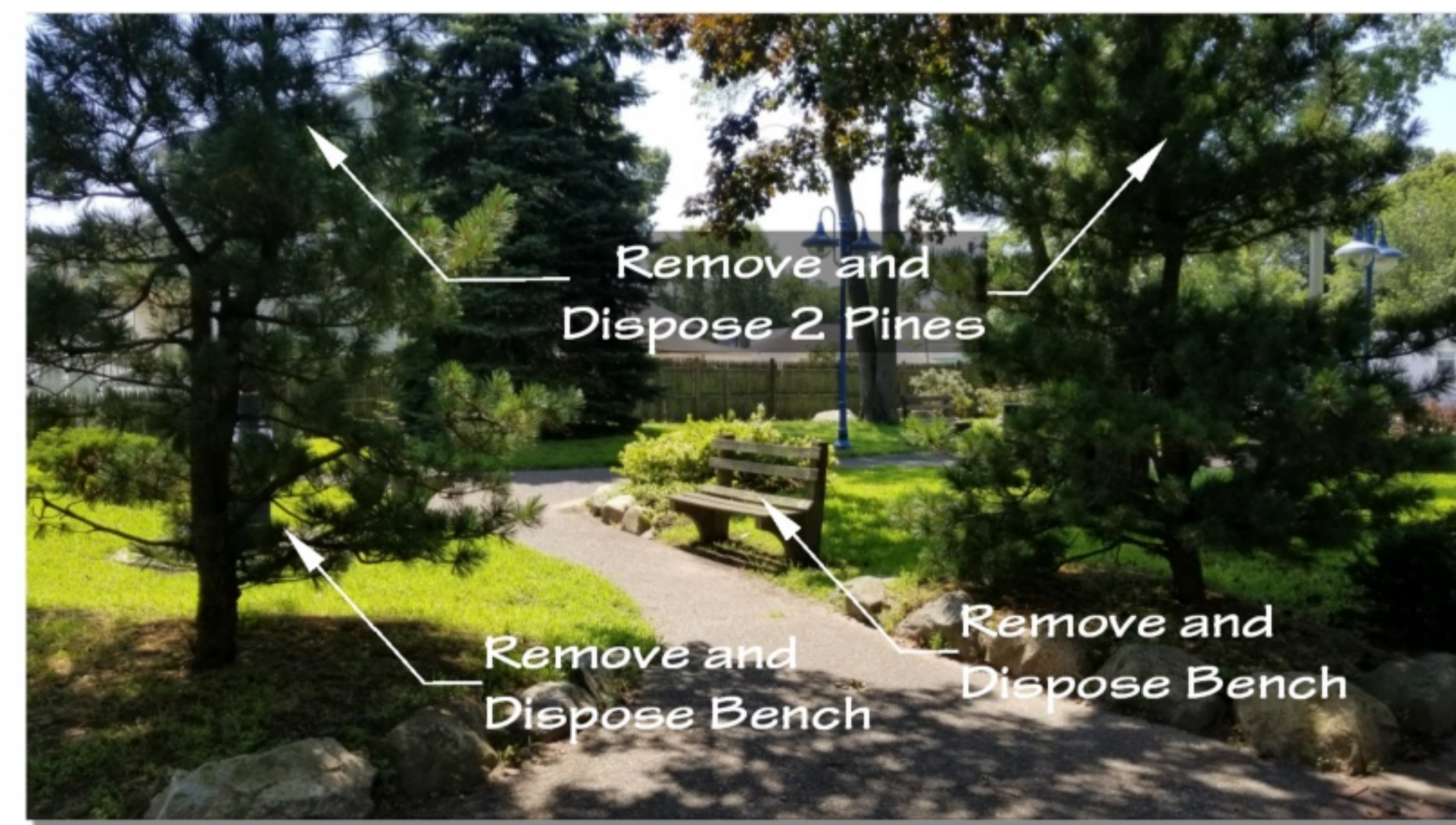
B Park entry at corner of Beach Avenue/ West Shore Road - Remove two (2) existing pine trees and two (2) existing benches along existing pathway including footings. Install one (1) 8' Dumor #58 black steel bench or approved equal.
