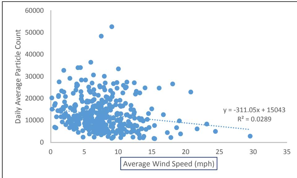
**Figure 5:** *Effect of Wind Speed on PC at Lydick Site*
