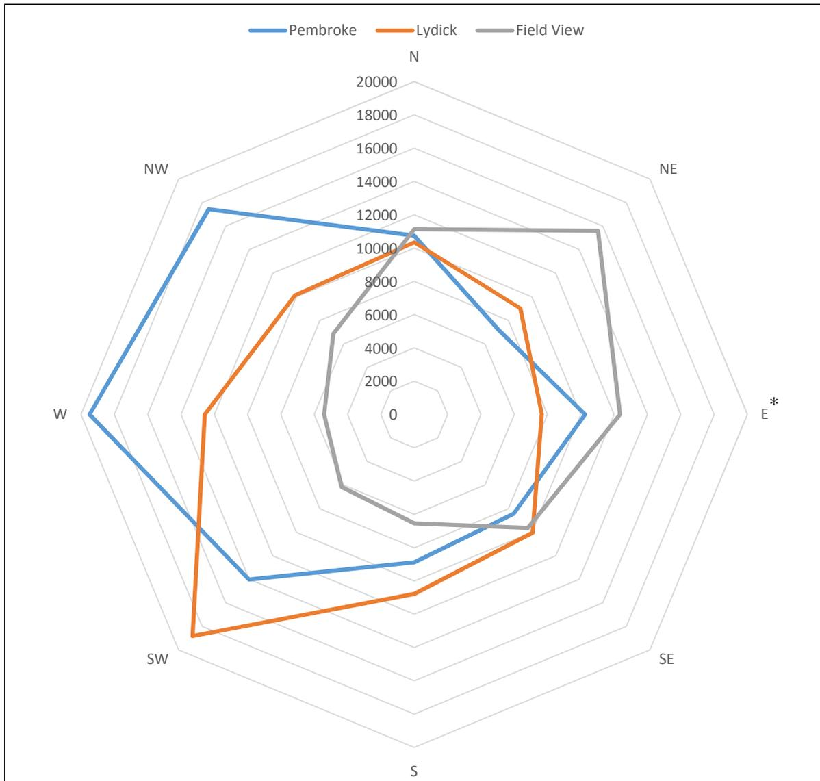
The average particle counts (PC) at each site are highest when the site is downwind of the airport. For instance, the airport is southwest of the Lydick site, and PC levels at that site are highest when the wind is from the southwest. The data from when the wind is from due east are not reliable, as the prevailing wind was only from that direction on three days.
