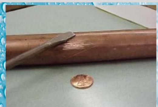
COPPER— scraping a copper pipe will reveal a shiny "new penny" color and will not attract a magnet. GALVANIZED IRON— Scraping a galvanized iron pipe will reveal a silver/white color and <u>will</u>attract a magnet.
